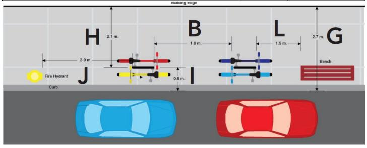
**STANDARD BIKE DIMENSIONS**: 0.6m Wide (Handle bars) x 0.8-1.2m Tall x 1.5-1.8m Long (Wheelbase)
